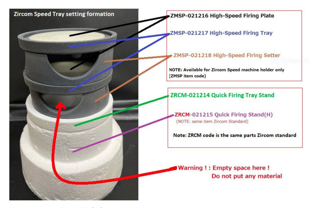
High Speed Firing Tray: Silicon carbide (SiC)compound form, If zirconia material touches this tray or there is no High Speed Firing Plate, it will change the color (light YELLOW). Please do not contact the SiC tray with zirconia material. Always should be put on the High Speed Firing Plate. Also, It can not be a cause of this tray itself to GRAY colored zirconia materials. exception: reduction firing CO concentration up 4% or please attempt other company's zirconia material.
